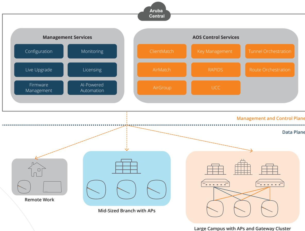
Figure 1. Distributed ArubaOS 10 supports APs and optional gateways.
