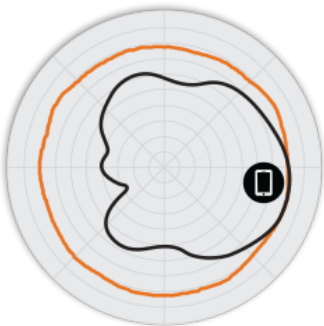
Figure 2. H320 2.4GHz Azimuth Antenna Patterns
