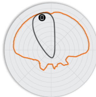
Figure 4. H320 2.4GHz Elevation Antenna Patterns
